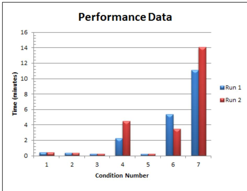
The results indicate the performance of `cvfsck -U <fsname>` to unmap thin provisioned LUNs varies significantly. Additionally, the unmap operations in the system continue for several seconds, as they continue to run in the background.
